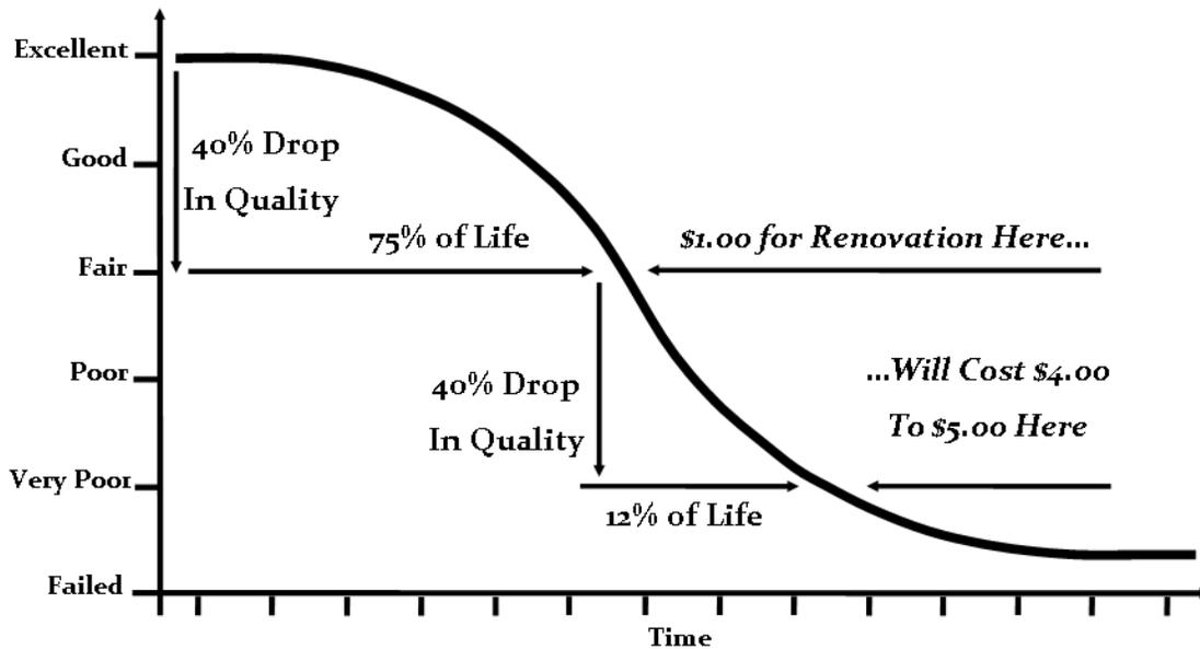
Figure VI-1. Pavement Deterioration Curve
